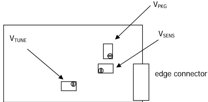
Figure 1. Potentiometers and associated voltages.
