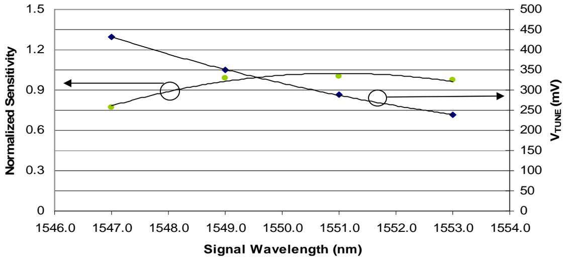
Fig. 2. Appropriate  $V_{TUNE}$  vs Signal Wavelength.
